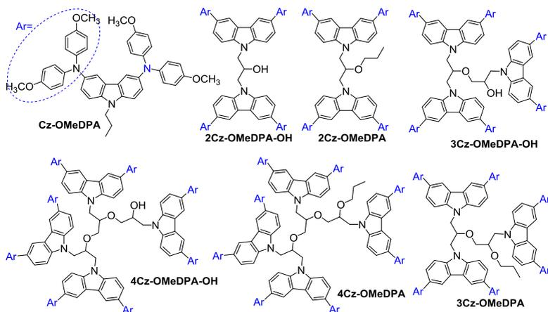
**Figure 1.** Chemical structures of synthesized organic semiconductors.
